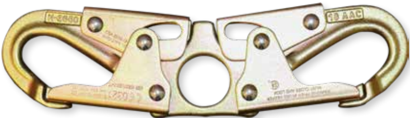
#274 Steel locking spreader snaphook, 3/4" gates Proof loaded up to 3,600 lbs. Minimum breaking load: 5,000 lbs.
