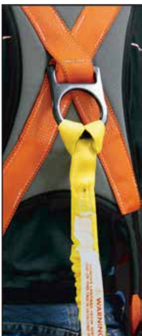
Choke-Loop 2 Internal shock absorber Looped end
