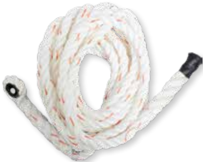
121-1T 5/8" rope lifeline Thimble on one end "Whipped" opposite end
