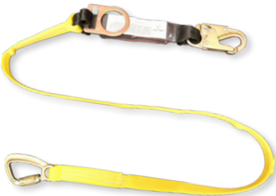
456AW-EXT #Z74 locking snaphook one end #63 (3/4" opening) auto locking snaphook other end Pack style shock absorber D-Ring for additional connections
