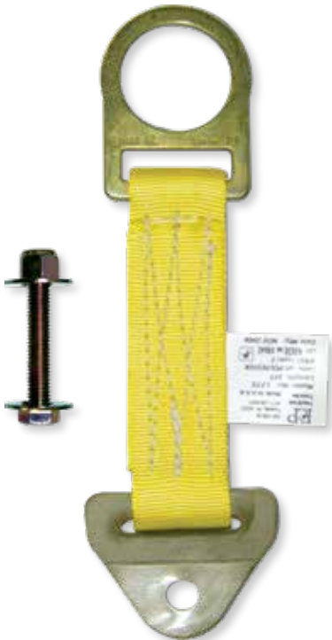
1775-S3 Steel anchor plate (Bolts to steel surfaces) 1/4" stainless steel anchor plate with, grade 8 bolt, nut, & washer 1 3/4" webbing with D-ring 1 3/4" maximum steel thickness
