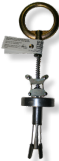
1770 3/4” portable/reusable concrete hole anchor Rated to 5,000 lbs Use for vertical and overhead concrete
