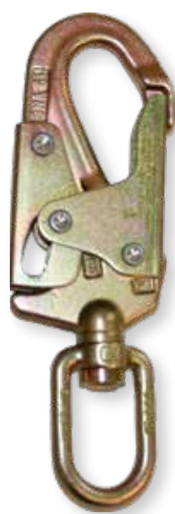
#49 Steel swivel locking snaphook, 3/4" gate Proof loaded to 3,600 lbs. Minimum. breaking load: 5,000 lbs.
