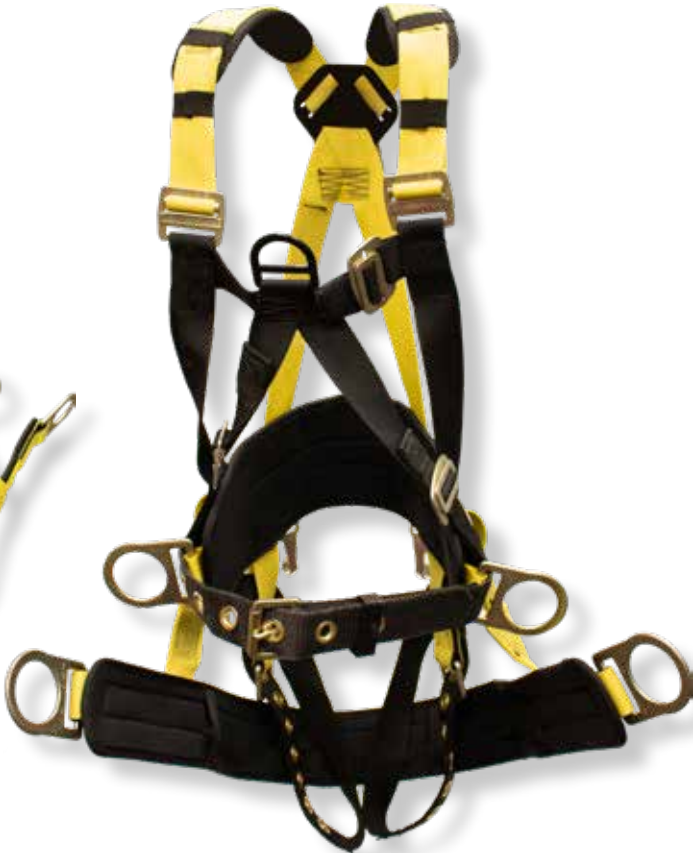
887PBT 6-point adjustment Adjustable sternum D-ring Back pad Accessory rings Fixed rigid suspension saddle Hip-positioning D-rings Tongue buckle/grommet legs
